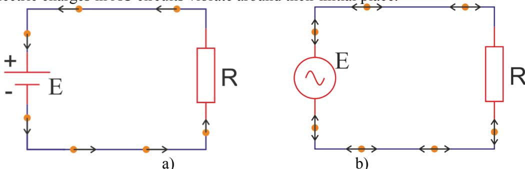
Fig. 5.2. Electron flow in DC (a) and AC (b) circuits
