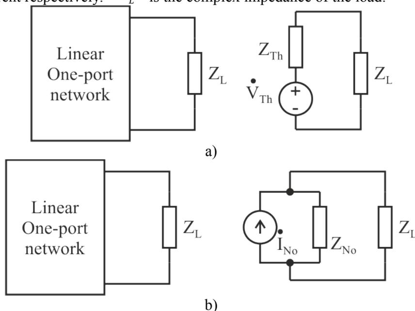
Fig. 5.34. Thevenin (a) and Norton (b) equivalent circuits.
