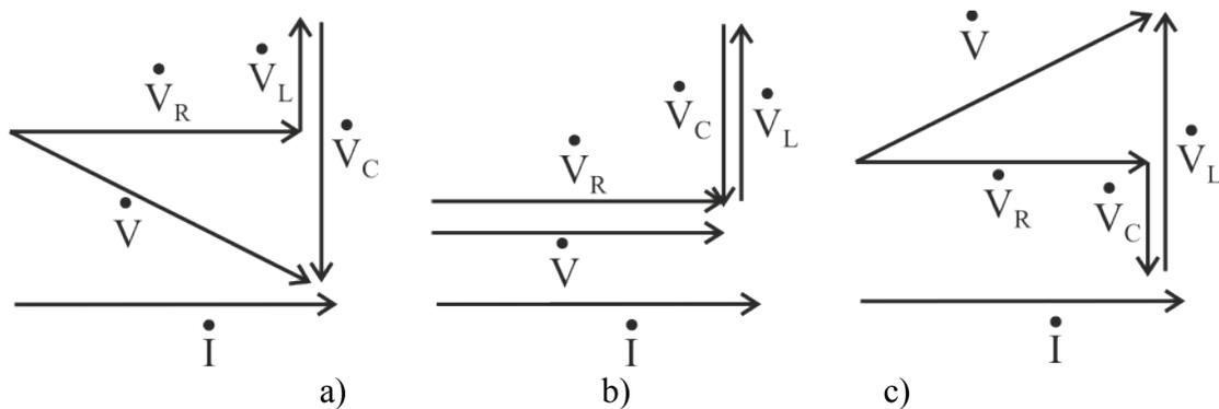
Fig. 5.14. Vector diagrams of a series RLC circuit: a)  $\frac{1}{\omega C} > \omega L$  ; b)  $\frac{1}{\omega C} = \omega L$  ; c)  $\frac{1}{\omega C} < \omega L$  .
