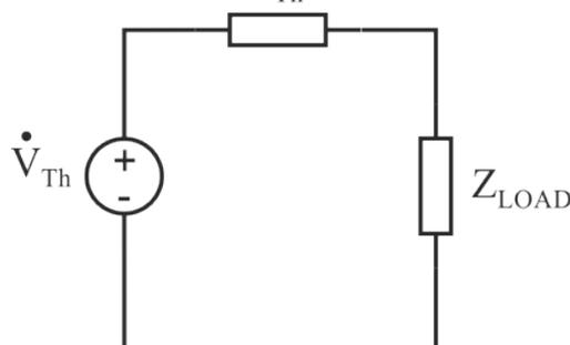
Fig. 5.27. Thevenin equivalent circuit powering a load.
