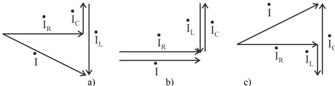
Fig. 5.17. Vector diagrams of a parallel RLC circuit: a)  $\omega C < \frac{1}{\omega L}$  ; b)  $\omega C = \frac{1}{\omega L}$  ; c)  $\omega C > \frac{1}{\omega L}$  .
