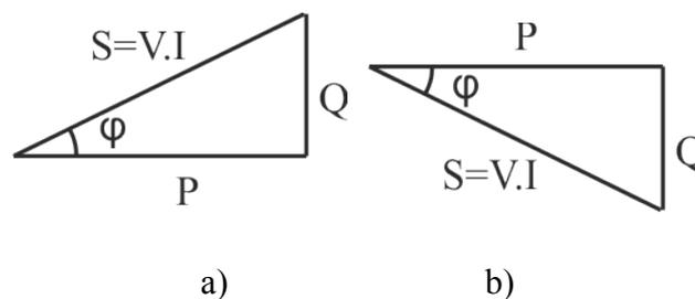
Fig. 5.26. Power triangle for: a) inductive load; b) capacitive load.
